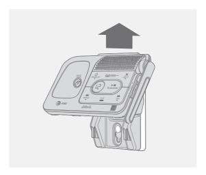
3. Unplug the telephone line cord or the DSL filter from the telephone wall jack. Push the telephone base up and away from the wall-mount bracket to detach it from the wall-mount bracket.
