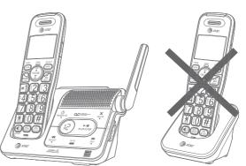
For registration, put the handset on the telephone base, not the handset charger.
