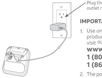
Plug the power adapter into a power outlet not controlled by a wall switch.
