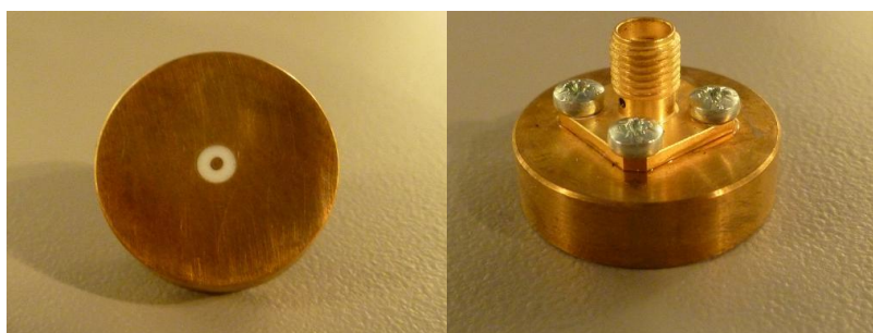
Figure 1 – MVG LIMESAR Dielectric Probe
