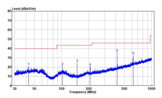
Site : chamber Condition: 3m VERTICAL Job No. : SZNS220607-24962E-RF Test Mode: PP Adapter : A318-060040W-US1
