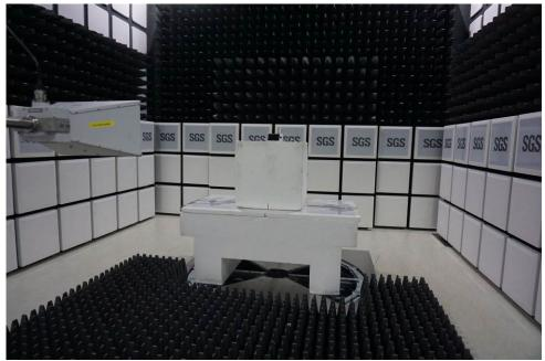
**Conducted RF Output Power Test Setup**
