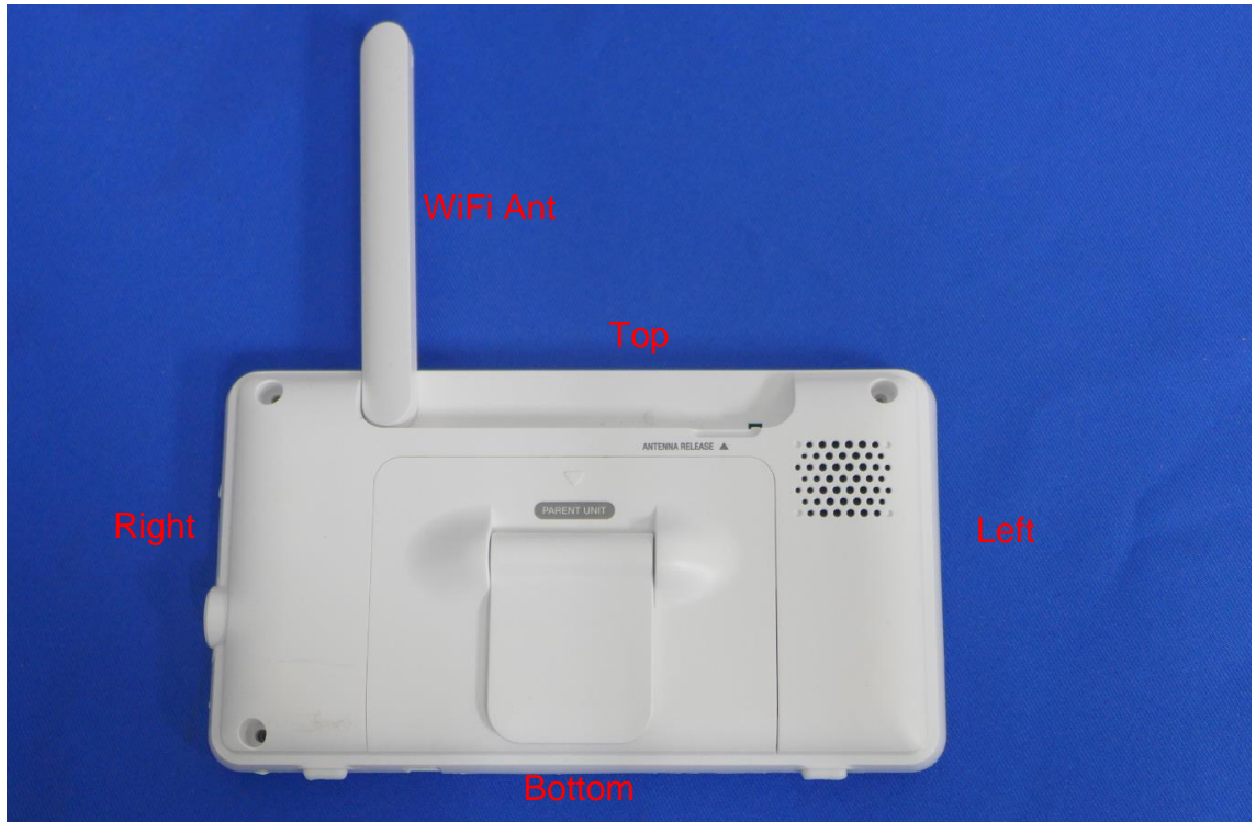
Photo 11: DUT Antenna Locations(Back View)
