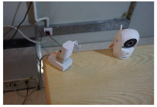
Radiated Emissions (30MHz-1GHz) Test Setup
