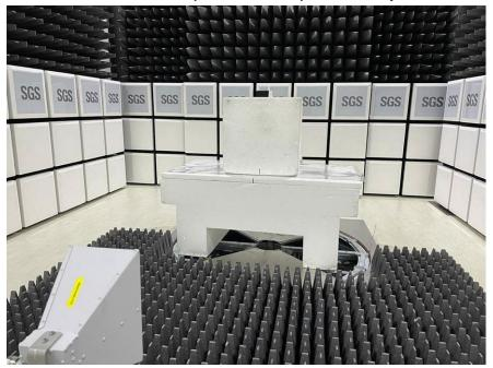
**Conducted RF Output Power Test Setup**
