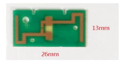
Figure 1 Physical dimension (mm)
