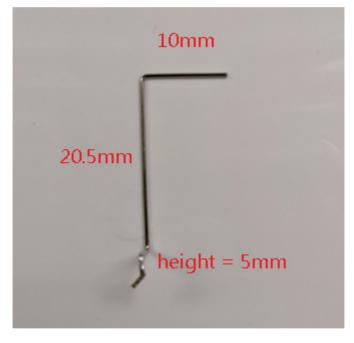
Figure 1 Physical dimension (mm)
