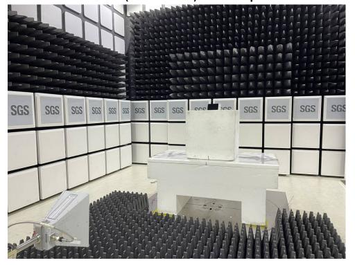
**Conducted RF Output Power Test Setup**
