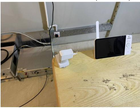
Radiated Emissions (30MHz-1GHz) Test Setup
