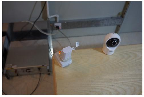
Radiated Emissions (30MHz-1GHz) Test Setup
