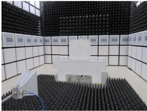
**Conducted RF Output Power Test Setup**
