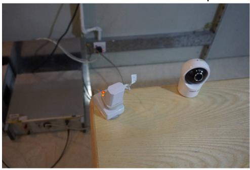
Radiated Emissions (30MHz-1GHz) Test Setup
