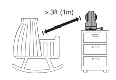
2. Adjust the angle of the camera to aim at your baby. Refer to the online help topics on how to use the Pan/tilt and Zoom functions of the camera
