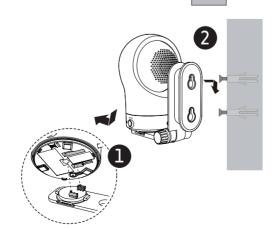
5. You can maximize your camera unit's viewing angles by tilting the wall mount bracket. Hold the camera unit, and then rotate the knob in anticlockwise direction. This will loosen the joint of the wall mount bracket. Tilt your camera unit up or down to adjust to your preferred angle. Then, rotate the knob in clockwise direction to tighten the joint and secure the angle.
