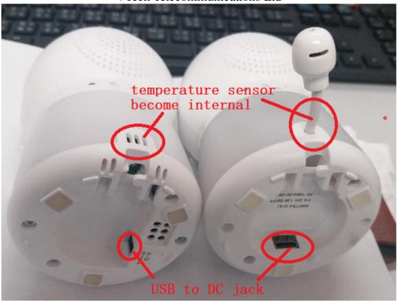
According to the changes above, just partial sensor and Power PCB layout interface were change, Hence, Conducted Disturbance at AC Power Line; Conducted Peak Output Power and Radiated Emission were re-evaluated, and then C2PC was requested in this application.
