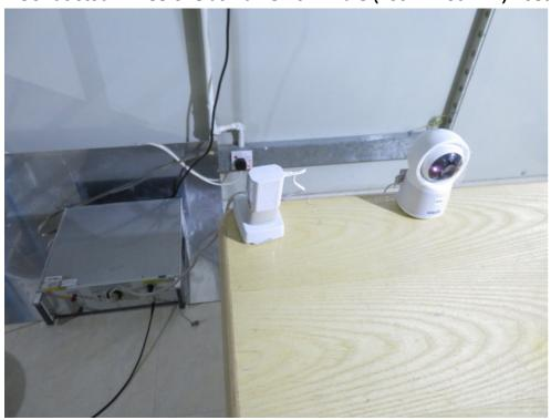
Radiated Emissions (30MHz-1GHz) Test Setup
