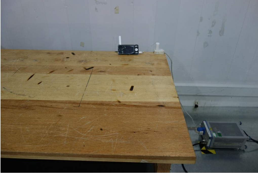
Conducted Disturbance at AC Power Line:
