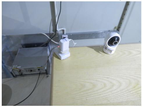
Radiated Emissions (30MHz-1GHz) Test Setup
