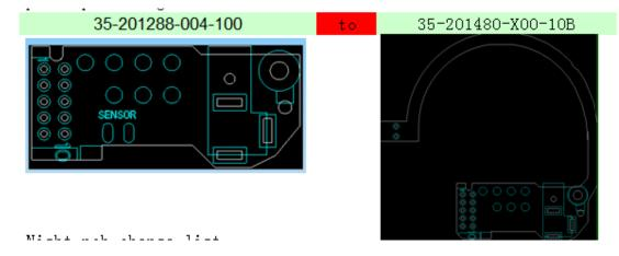
3.The PCB layout of Night Light was changed from surface Mounted technology component to through hole technology component, And the circuit was changed as from A (35-201287-X04-10A to B (35-201480-X00-10A). And the LED component from "19-217/S2C-AM2N2VY/3T(V) \_LED5,LED6,LED7 " and 19-217/G7C-AP1Q2B/3T\_LED1,LED4,LED8" to "YL5ARGB9UCK22/P17-H,\_LED2,LED6,LED7".
