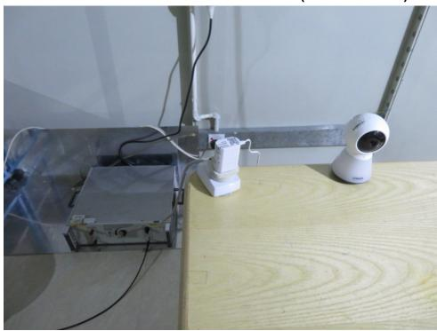
Radiated Emissions (30MHz-1GHz) Test Setup
