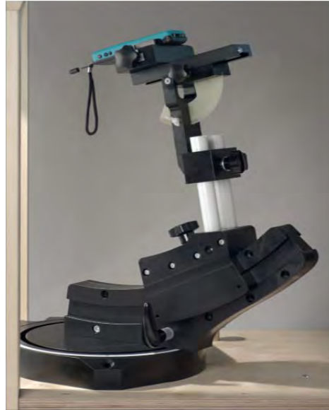
F-2. Device Holder for Transmitters
