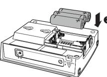
Match the polarity markings (+ and -) inside the battery compartment
