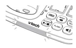
2. <u>Press and hold</u> **W** on the remote ringer until the green LED light on the remote ringer flashes, then release 🏜
