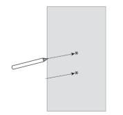
2. Drill two holes in the wall (7/32" drill bit). If you drill the holes into an object other than a stud, insert the wall anchors into the holes and tap gently on the ends with a hammer until the wall anchors are flush with the wall.
