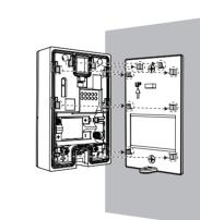
2. Push the doorbell gently onto the wall mount cover until they are sealed tightly.
