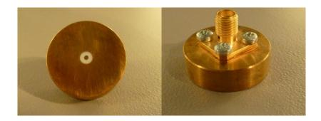
**Figure 1** – *MVG LIMESAR Dielectric Probe*
