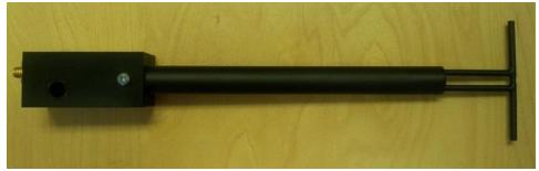
**Figure 1** – *MVG COMOSAR Validation Dipole*
