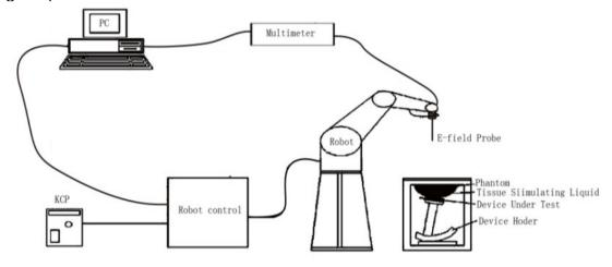
Figure 1: Schematic diagram of the SAR measurement system
