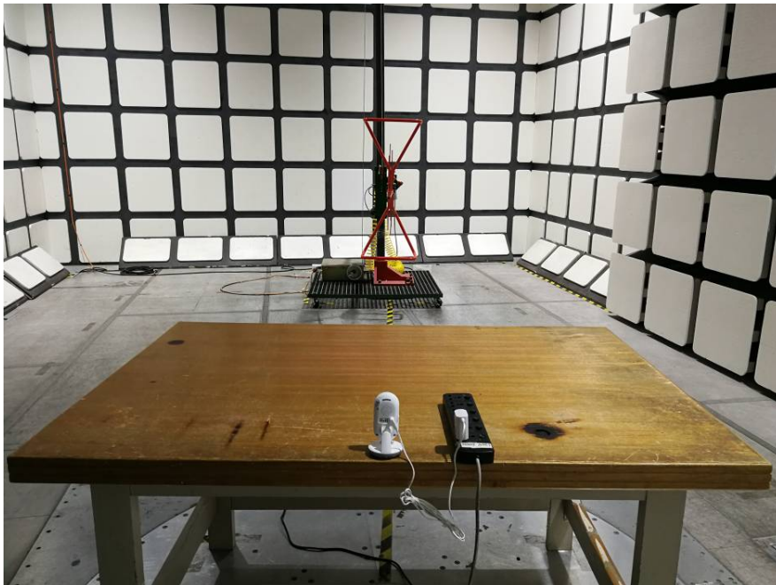
Radiated Emissions View (Above 1 GHz)
