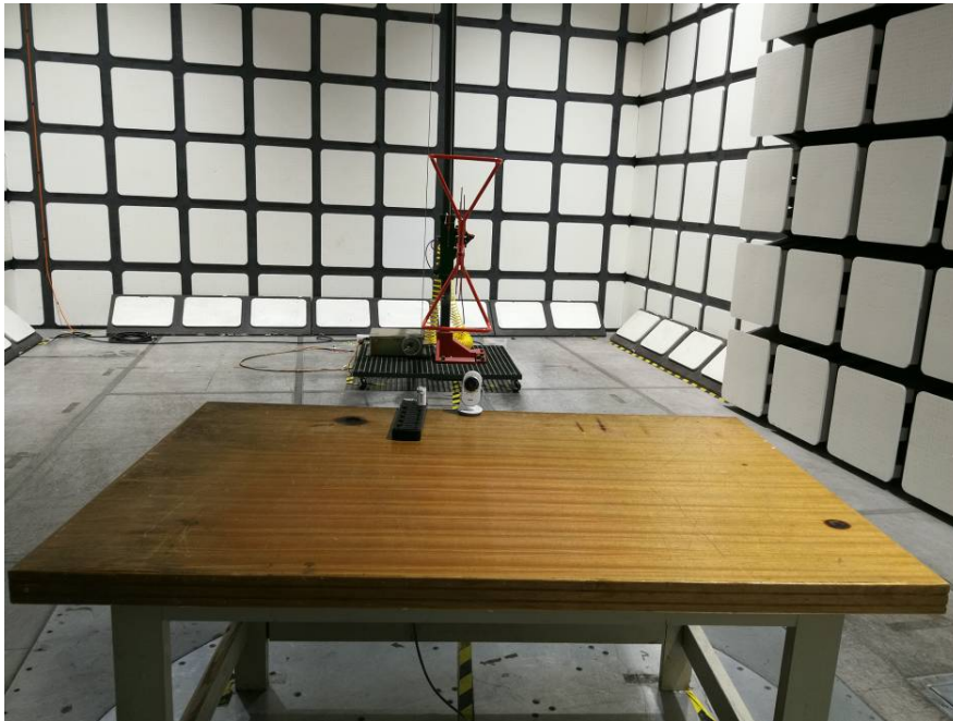
Radiated Emissions View (Below 1 GHz)
