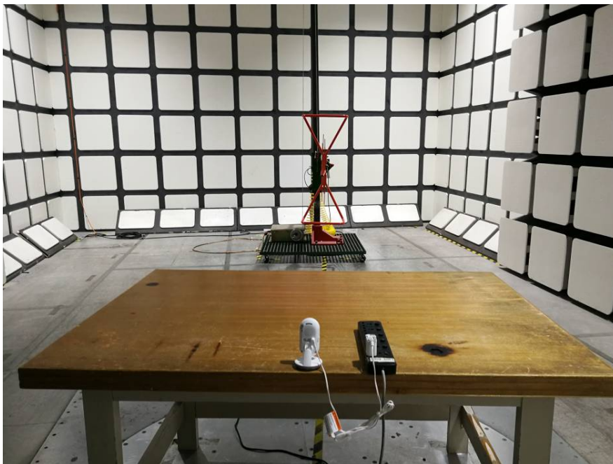
Radiated Emissions View (Above 1 GHz)
