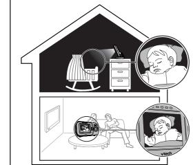
The baby unit has infrared LEDs that allow you to see your baby clearly at night or in a dark room. When the baby unit being viewed detects low light levels, the infrared LEDs are switched on automatically. The images from the baby unit are in black and white, and 🕽 appears on the screen.
