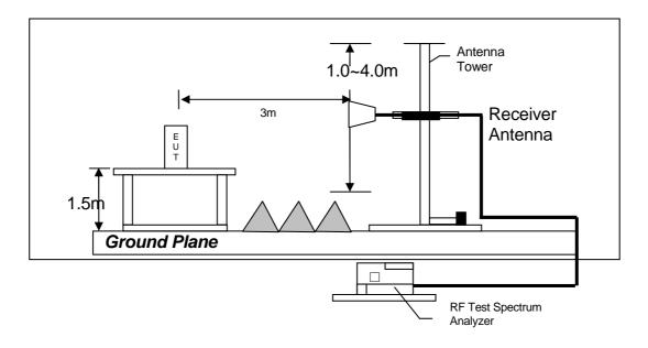
Test setup of radiated emissions above 1GHz
