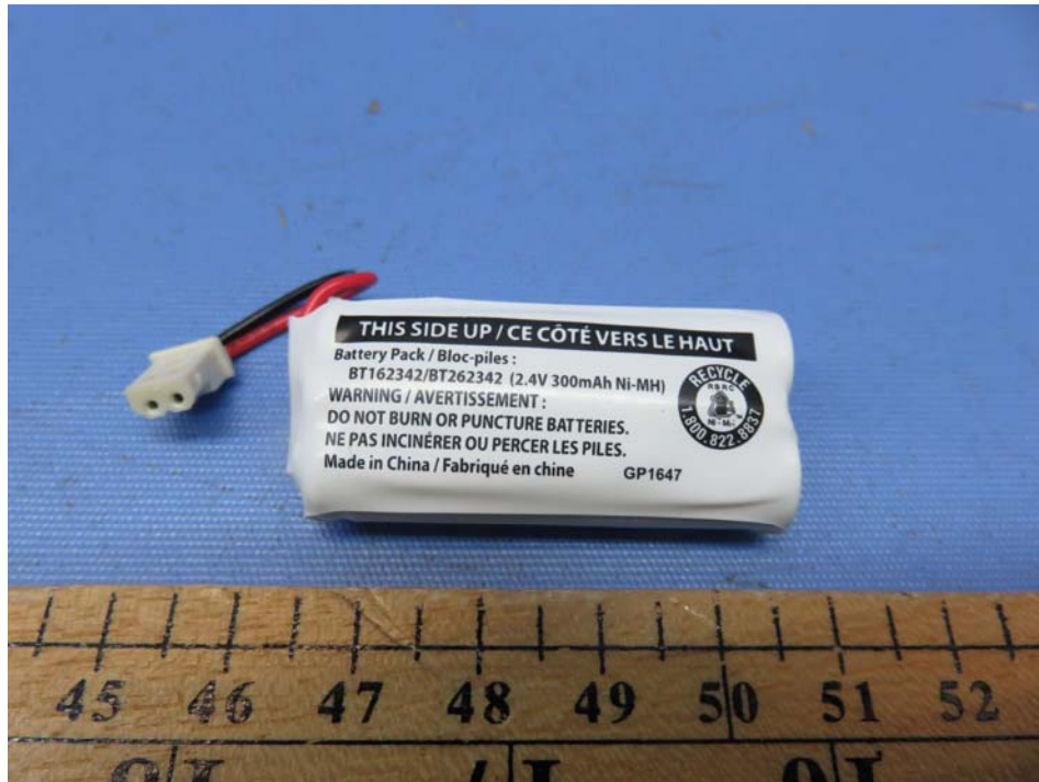
Figure 3 – 2.4V 300mAh GPI rechargeable battery pack
