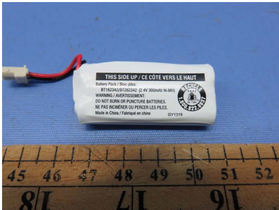
Figure 4 – 2.4V 300mAh Coslight rechargeable battery pack
