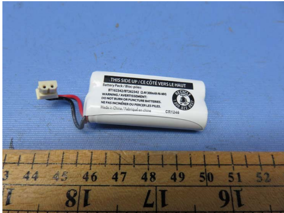
Figure 5 – 2.4V 300mAh Corun rechargeable battery pack
