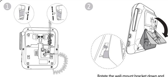
Press the tabs of the wall-mount bracket to release it from the tabletop orientation.
