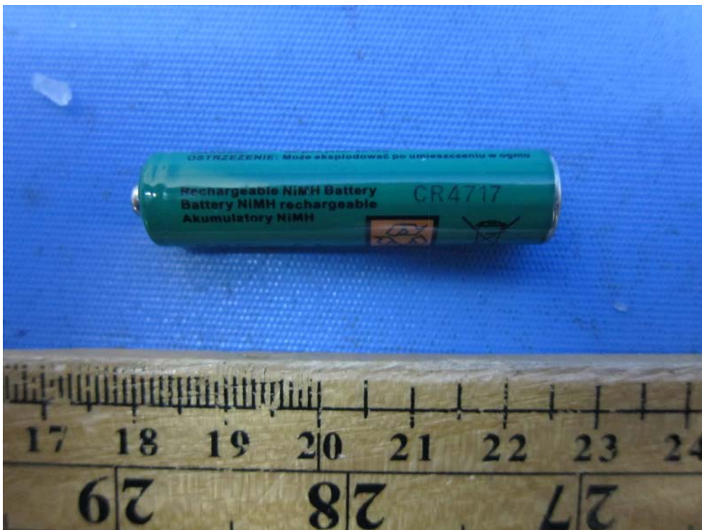
Figure 4 – 1.2V 500mAh Courn Ni-MH rechargeable battery
