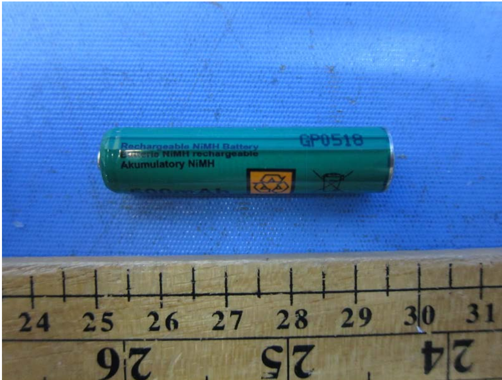
Figure 3 – 1.2V 500mAh GPI Ni-MH rechargeable battery
