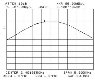
Max. Radiated Output Power Low Band - Ch. 0 Base Station 3 Meters Antenna Factor = 36dB Pt = 122dBuV
