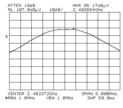
Max. Radiated Output Power High Band - Ch. 94 Base Station 3 Meters Antenna Factor = 36dB Pt = 121.2dBuV
