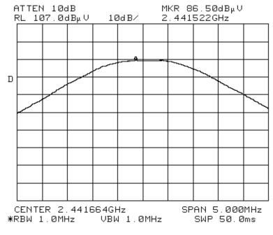
Max. Radiated Output Power Mid Band - Ch. 47 Base Station 3 Meters Antenna Factor = 36dB Pt= 122.5dBuV
