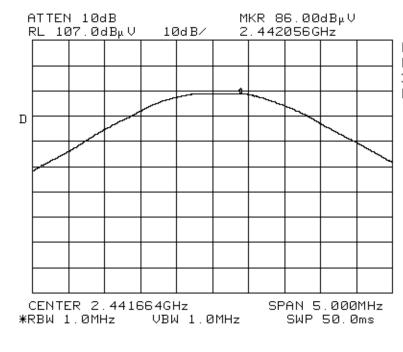
Max. Radiated Output Power Mid Band - Ch. 47 3 Meters Portable Antenna Factor = 36dB Pt= 122dBuV
