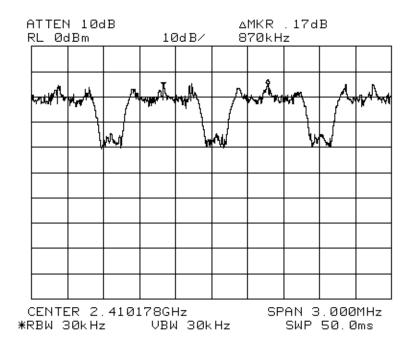
CH. Separation =870Khz Portable Hopping "On"
