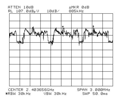
CH. Separation =885Khz Base Station Hopping "On"
