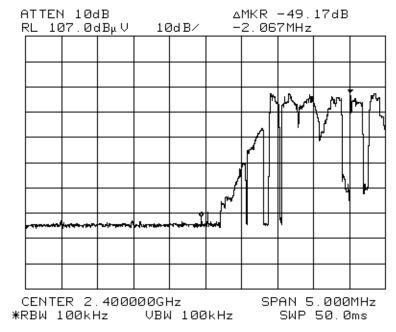
Lower Band Edge Emission Base Station Hopping "On"
