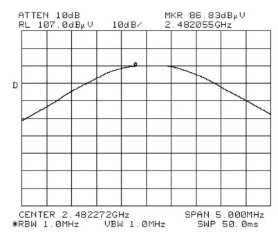
Max. Radiated Output Power High Band - Ch. 94 Portable Antenna Factor = 36dB Pt= 122.83dBuV
