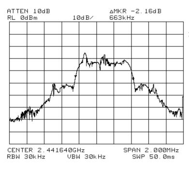
Portable 20dB Occ.BW = 663Khz Mid Band - Ch. 47
