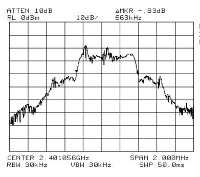
Portable 20dB Occ BW. = 663Khz Low band Ch. 0
