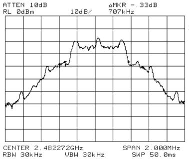
Base Station 20dB Occ.BW = 707Khz High Band - CH. 94
