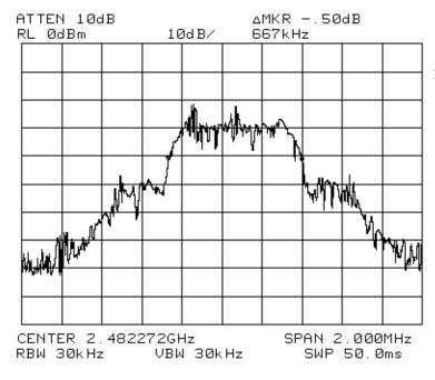
Portable 20dB Occ.BW = 667Khz High Band - Ch. 94
