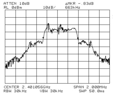
Portable 20dB Occ BW. = 663Khz Low band Ch. 0
