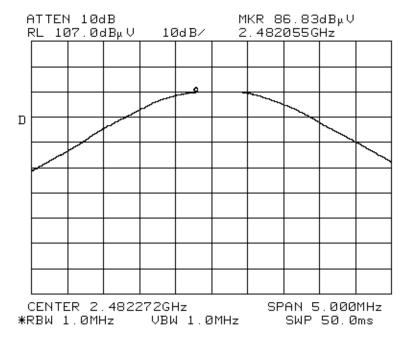
Max. Radiated Output Power High Band - Ch. 94 Portable Antenna Factor = 36dB Pt= 122.83dBuV
