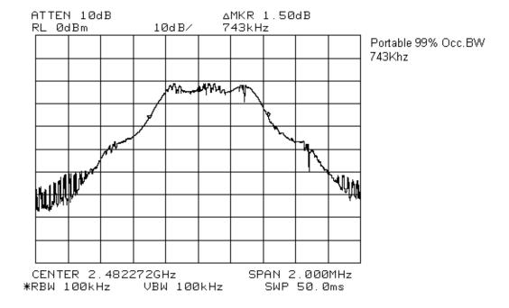
FCC PART 15, SUBPART C FREQUENCY HOPPING TRANSMITTERS PROJECT NO.: 1W03875
