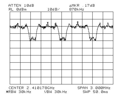
CH. Separation =870Khz Portable Hopping "On"
