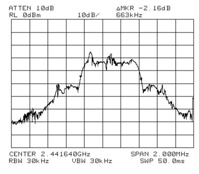
Portable 20dB Occ.BW = 663Khz Mid Band - Ch. 47
