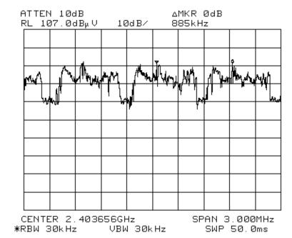
CH. Separation =885Khz Base Station Hopping "On"
