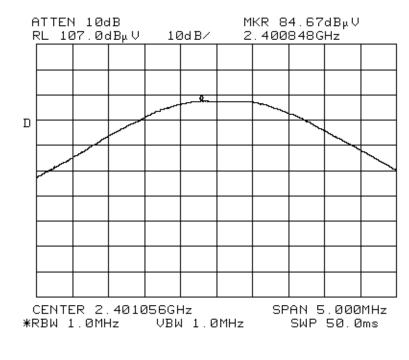
Max. Radiated Output Power Low Band - Ch. 0 3 meters Portable Antenna Factor = 36dB Pt= 120.7dBuV
