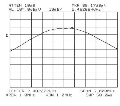
Max. Radiated Output Power High Band - Ch. 94 Base Station 3 Meters Antenna Factor = 36dB Pt = 121.2dBuV
