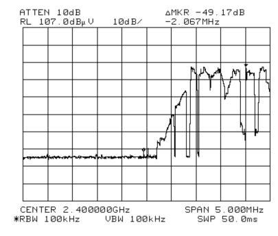
Lower Band Edge Emission Base Station Hopping "On"
