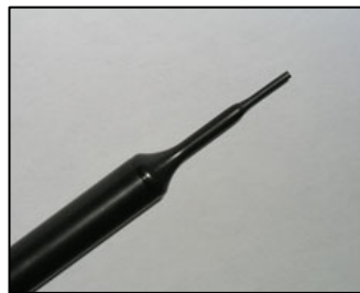
EX3DV4 E-field Probe
