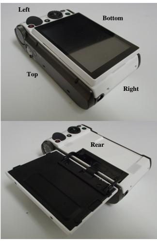
For Rear position, test was performed with LCD panel opened because it was nearer to antenna than that of LCD panel was closed.
