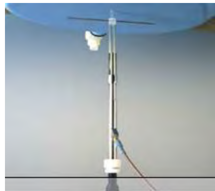
Photograph of the dipole Antenna
