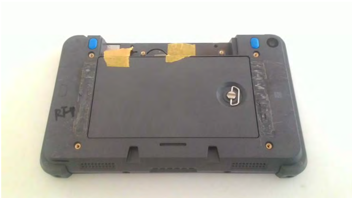
Fig.7 Back view of EUT (remove scanner and rails for SAR testing via KDB inquiry)
