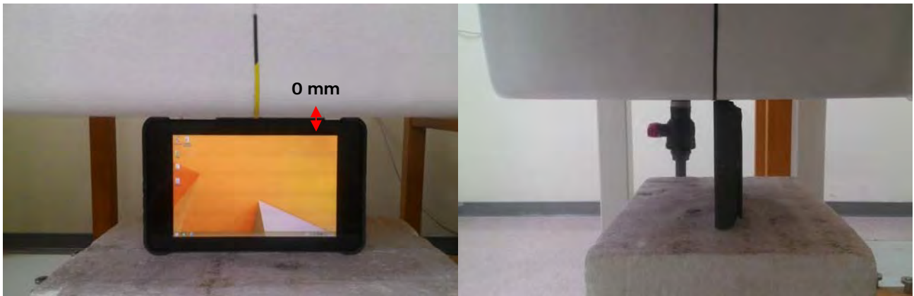
Fig.4 EUT Top side to flat phantom
