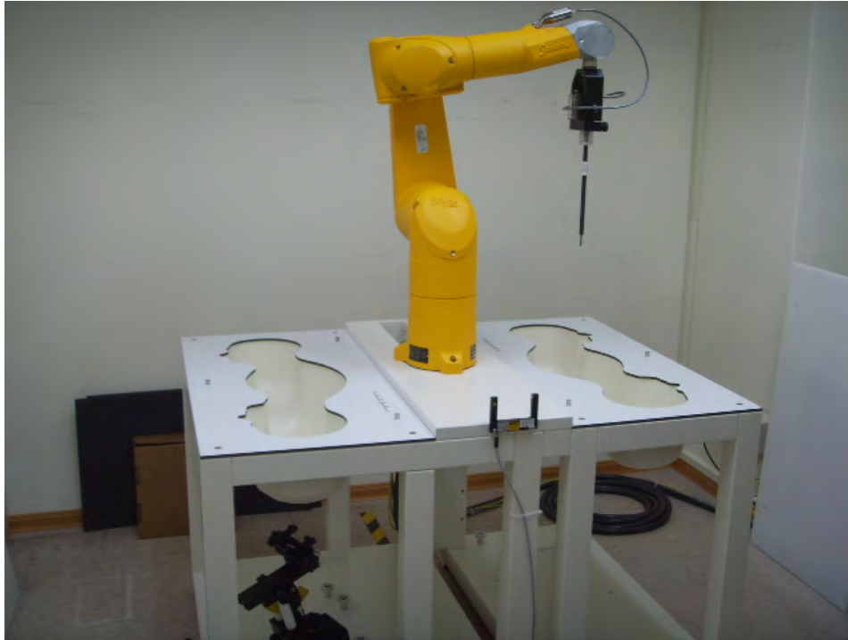
Fig.1 Photograph of the SAR measurement system
