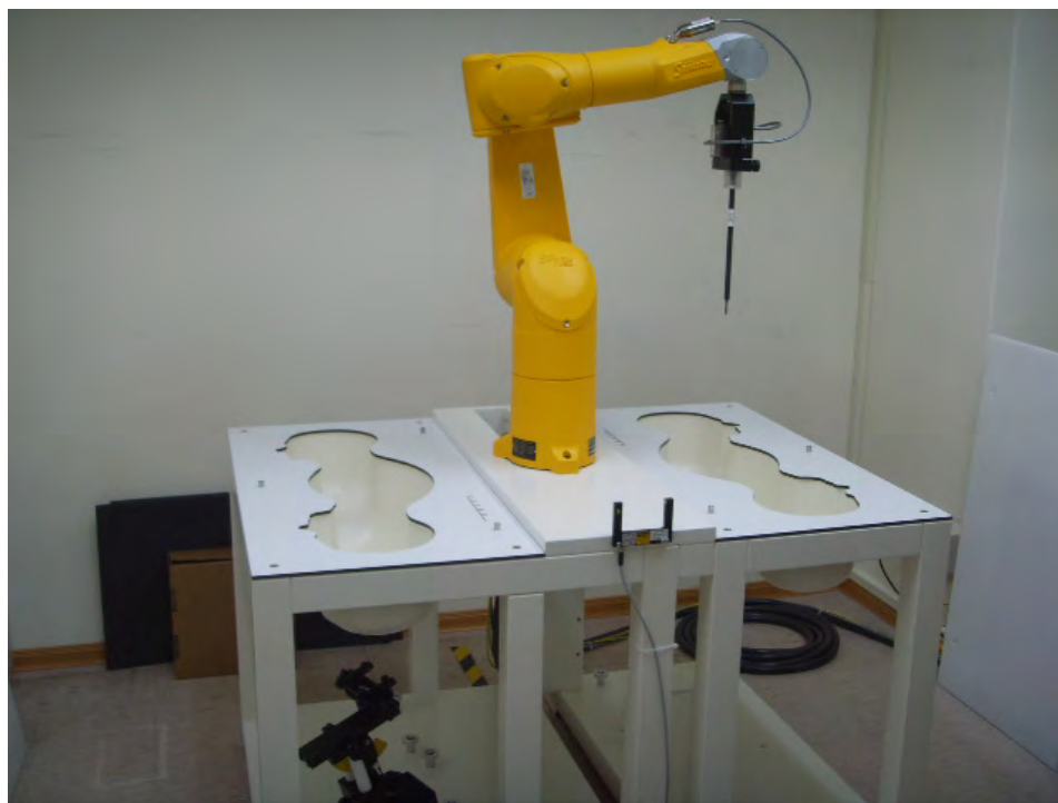
Fig.1 Photograph of the SAR measurement system
