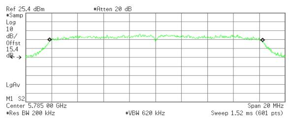
Occupied Bandwidth 16.4164 MHz Occ BW % Pwr 99.00 % x dB -26.00 dB
