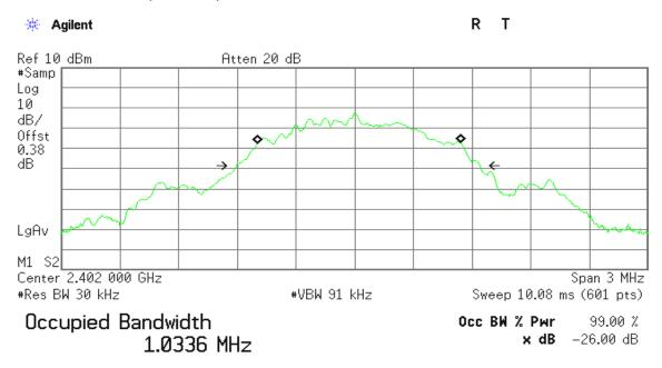
Transmit Freq Error 20.847 kHz x dB Bandwidth 1.247 MHz\*
