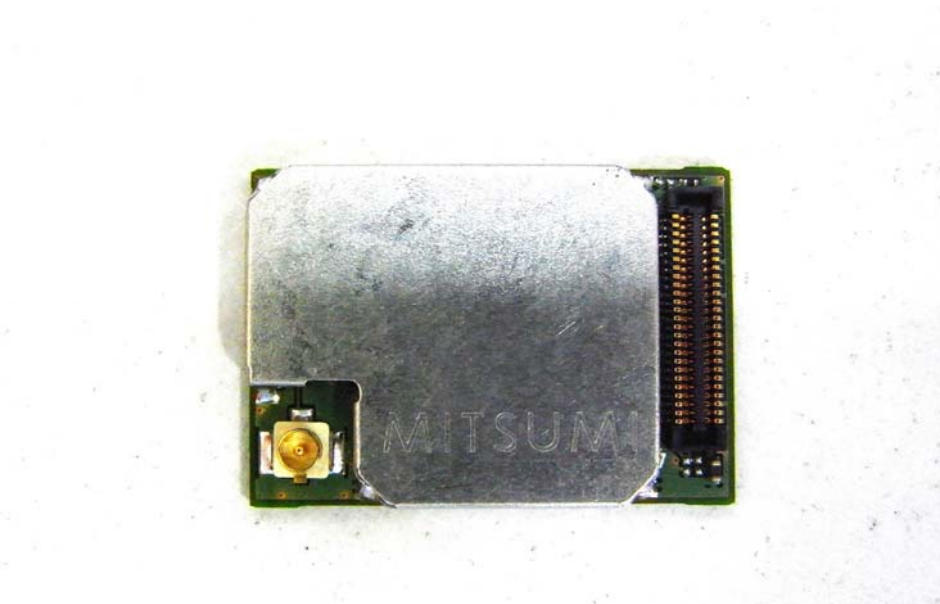
Top view (RF module with shield)
