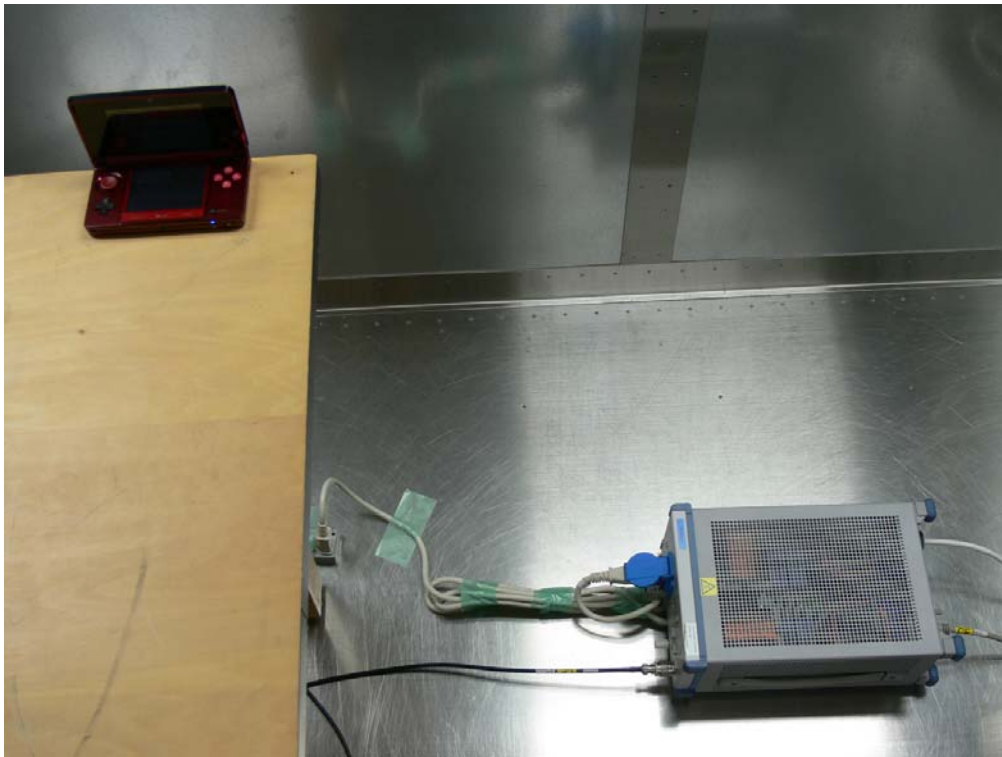
Photograph 1: Set-up for AC Mains Conducted Emission of Transmitter and Receiver, Front View
