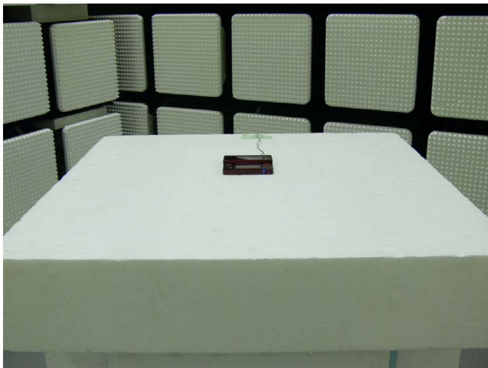
Photograph 5: Set-up for Radiated Emission, EUT Configuration Z-Axis (Movable antenna)
