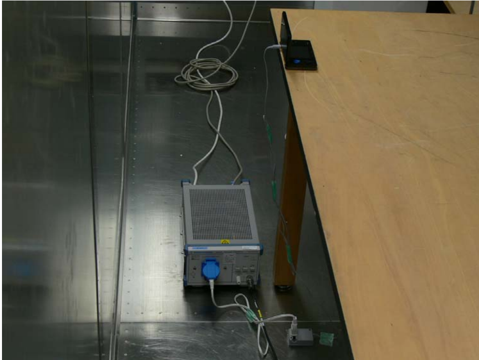
Photograph 2: Set-up for AC Mains Conducted Emission of Transmitter and Receiver, Rear View
