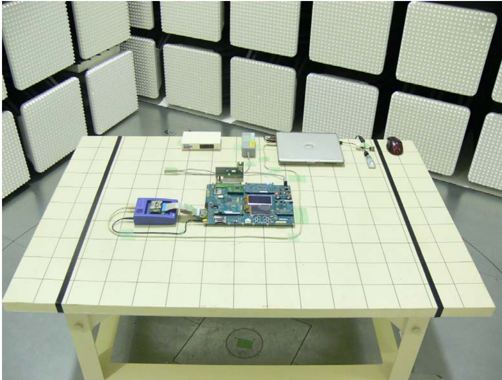
Photograph 6: Set-up for Radiated Emission, EUT Configuration X/Y-Axis
