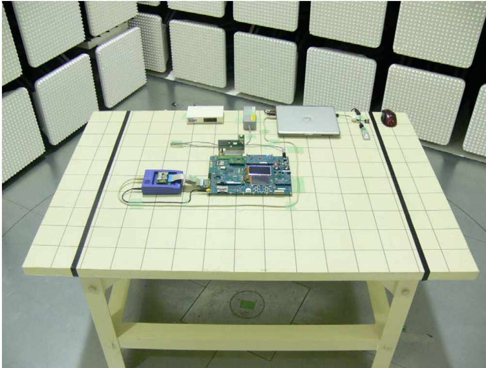
Photograph 8: Set-up for Radiated Emission of Transmitter, Front View
