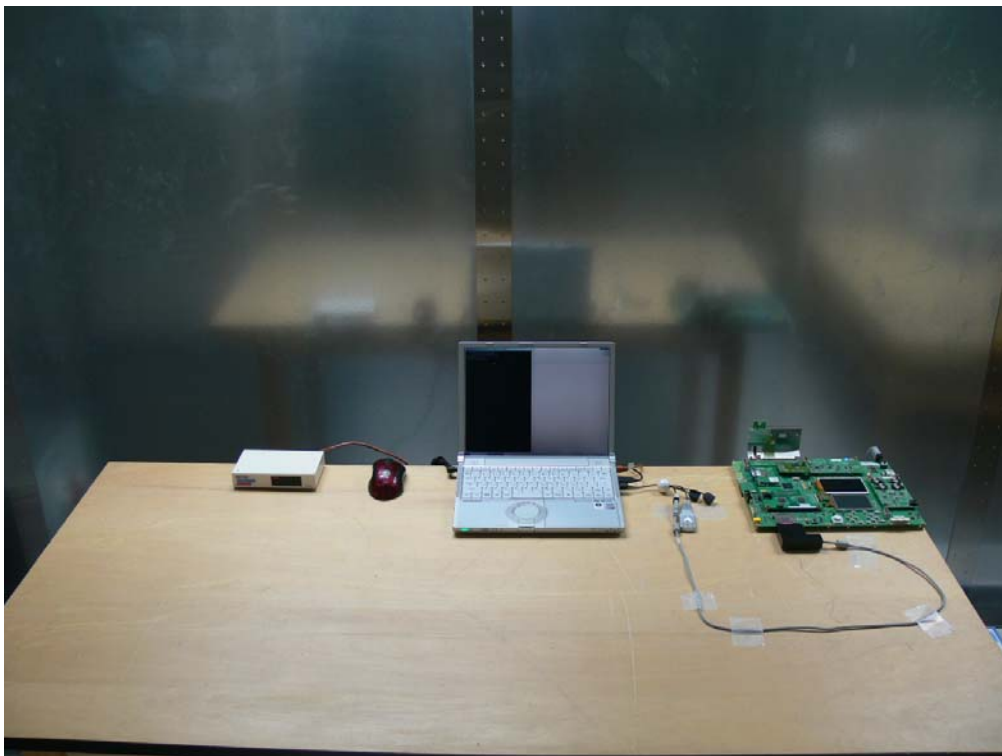
Photograph 3: Set-up for AC Mains Conducted Emission of Transmitter (802.11.b/g), Front View
