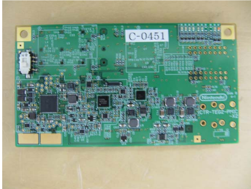
Top view (Nintendo DS CTR TARGET BOARD / Power Management IC part)
