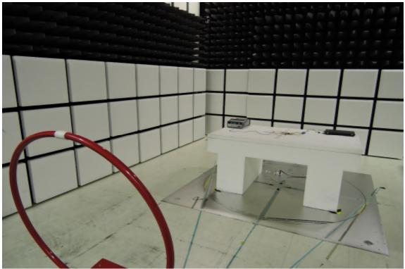
Radiated Emission Set up Photos (Below 1GHz)
