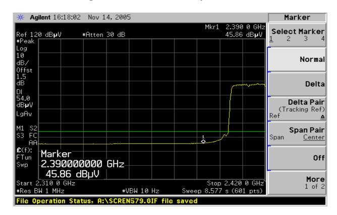
Detector mode: Peak Polarity: Horizontal
