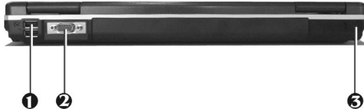
1. USB 2.0 Ports 2. VGA Port 3. Kensington Lock Hole
