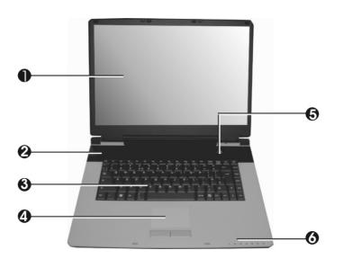
1. Color Widescreen LCD Display2. Built-in Stereo Speaker3. Keyboard4. Touchpad Pointing Device5. Power On/Resume Button6. LED Indicators
